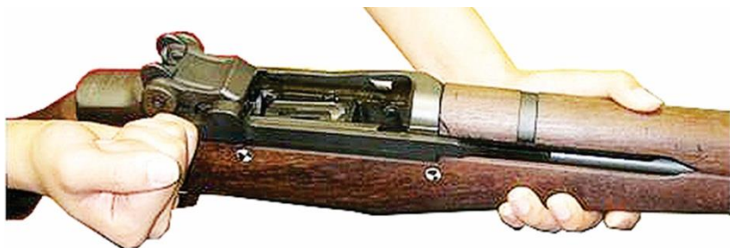
Figure 8. Checking that weapon is clear
