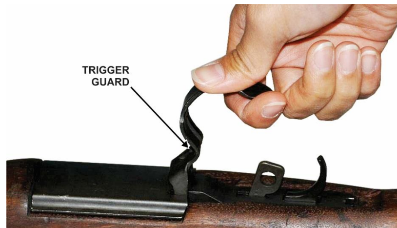
Figure 11. Trigger guard being pulled rearward and upward
