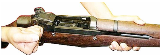
Figure 1. Pulling operating rod
