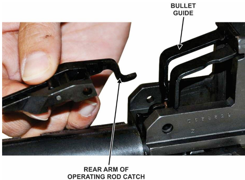
Figure 43. Rear arm of operating rod catch
