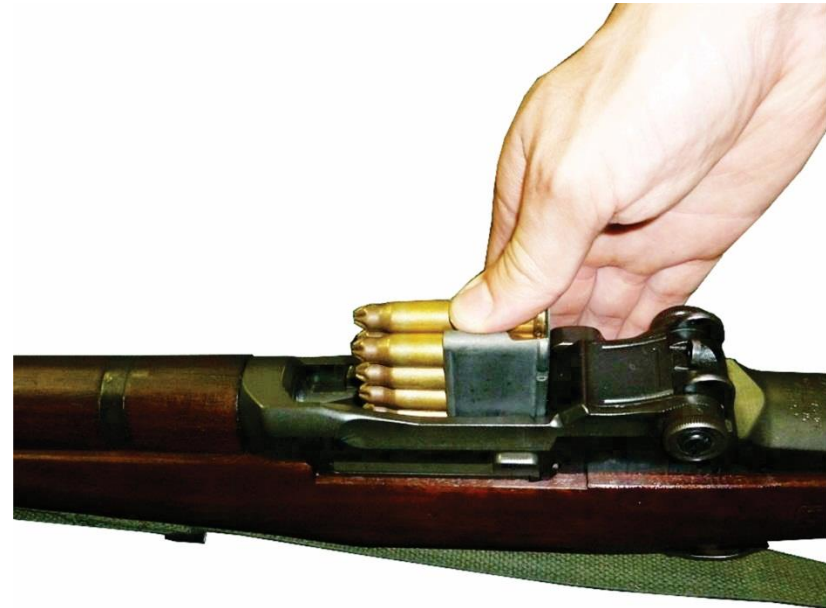
Figure 56. Loading of clip into rifle
