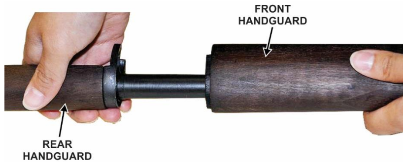
Figure 28. Removal of front handguard
