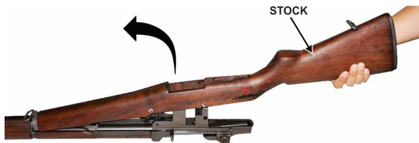
Figure 13. Lifting up stock
